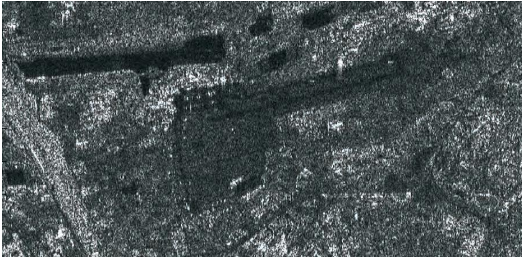
Figure 11: speckle on the image of Linate Airport, from (Ferretti, Monti-Guarnieri, Prati, & Rocca, February 2007)
